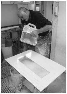
The pulp is precisely made into a slurry that "feels right" so it can be sprayed. A single sheet of our paper consists of wire mesh laminated between two layers of sprayed cotton pulp. The paper is set to dry, then completely sealed and painted with acrylics, Venetian plasters and thin layers of glaze.
